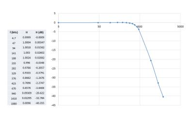
0.05% deviation at 50 kHz, 0.5% deviation at 250 kHz, -3 dB at 450 kHz, -22 dB at 1 MHz
